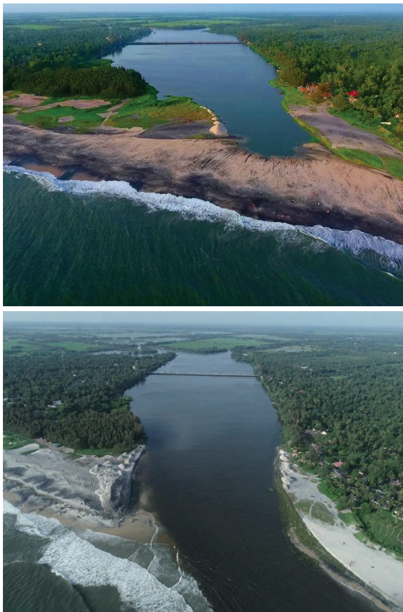
Figure 25 Aerial photographs of the sea mouth at the Thottappally Spillway, with the sand bar and after the manual removal of the sand bar during the floods of 2019.
