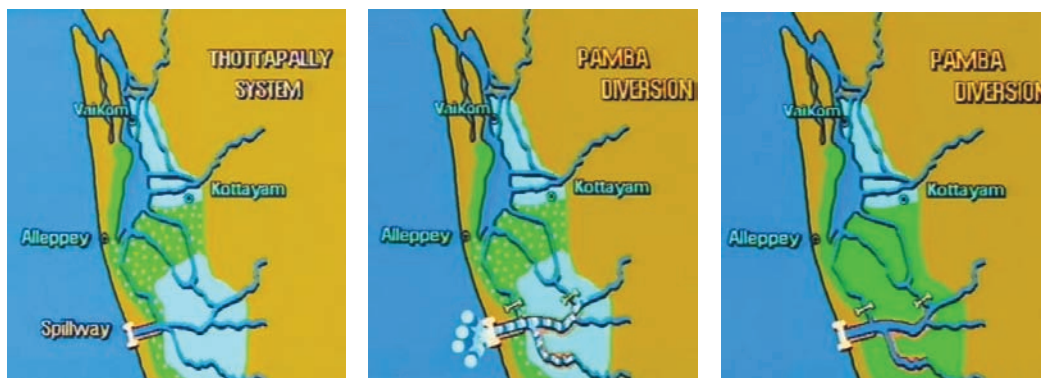
Figure 9 Pictorial description of the proposal for Pamba Diversion Scheme, Indo-Dutch Mission, Kuttanad
