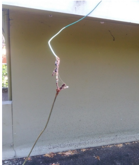
Picture 4.25: Shows the Low Quality Earth Wire Distributed by the Agency
