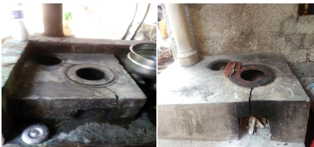
Picture 4.3.11 & 4.3.12: Chulhas which are Not Used by the Beneficiaries due to Cracks Developed
