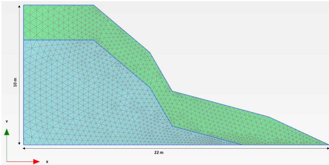
**Fig. 4.23:** Finite element mesh discretization of slope considered for the numerical model for Munnar Silent Valley Road site (LS1)
