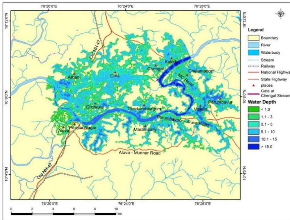
**Fig. 5.13:** Map showing the maximum depth of inundation corresponding to a 24h 100-year rainfall with an initial storage of 85% in the reservoirs and with the provision of a flow regulator at Chengal Stream and Periyar River confluence.
