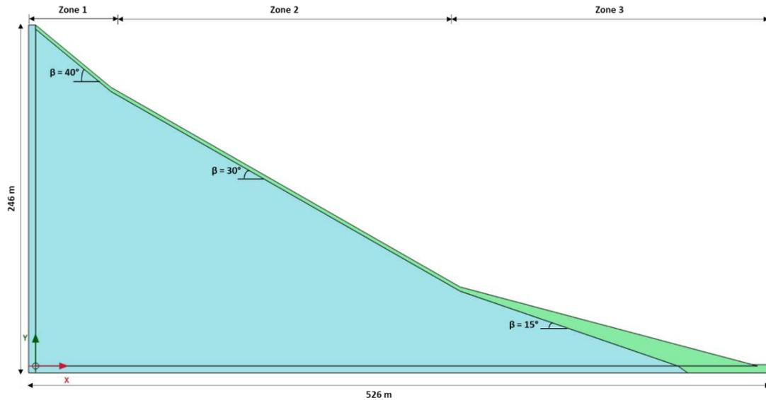
**Fig. 4.13:** Input geometry of slope in the numerical model at Kavalappara site of Malappuram district
