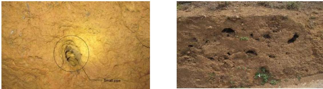
**Fig. 4.3:** A small pipe formed in the soil column (left); soil-piping affected region (right)
