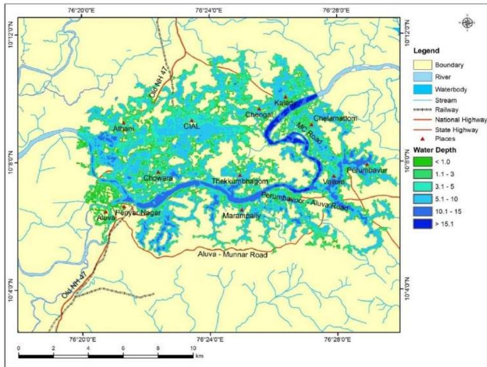
**Fig. 5.11:** Map showing the maximum depth of inundation corresponding to a 24h 100-year rainfall with an initial storage of 85% in the reservoirs.
