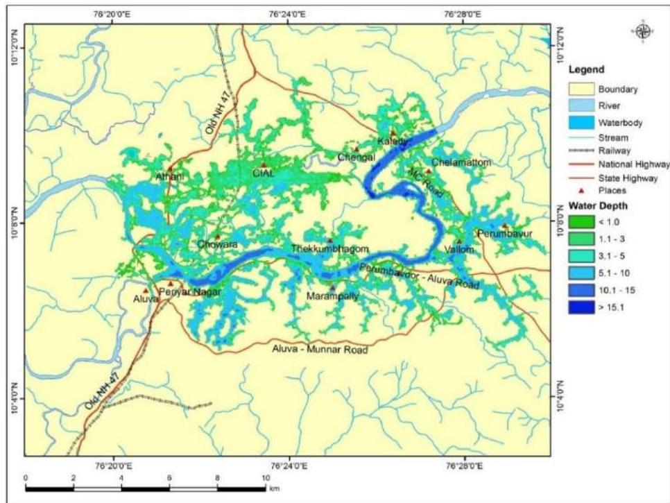
**Fig. 5.9:** Map showing the maximum depth of inundation corresponding to a 24h 100-year rainfall with an initial storage of 50% in the reservoirs.
