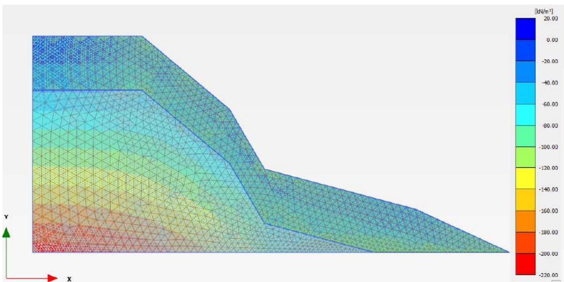
**Fig. 4.24:** Estimated geostatic stresses ( $\sigma_{yy}$  - vertical effective stress) in the FEM model - Initial phase for Munnar Silent Valley Road site (LS1)
