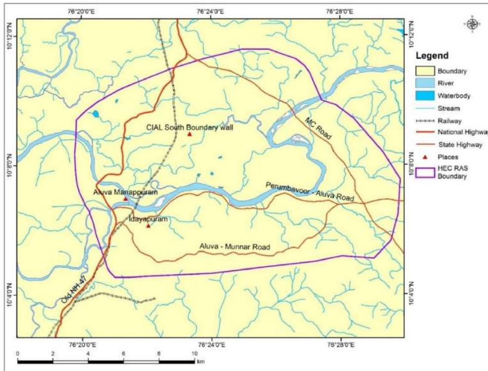
**Fig. 5.8:** Map showing portion of the Periyar River considered for flood inundation modelling using HEC RAS
