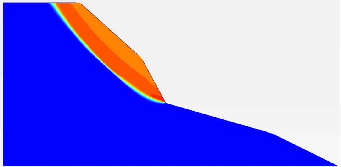
**Fig. 4.25:** FEM model, incremental displacement contours at the time of failure (fully saturated) – Case 3 ( $FoS < 1$ ) for Munnar Silent Valley Road site (LS1)
