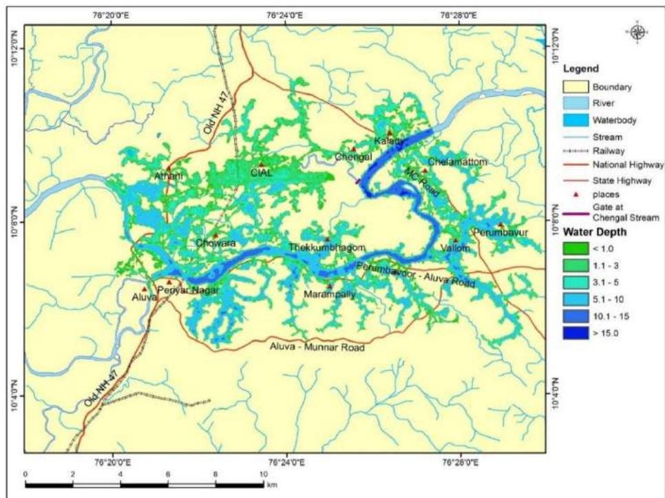
**Fig. 5.12:** Map showing the maximum depth of inundation corresponding to a 24h 100-year rainfall with an initial storage of 50% in the reservoirs and with the provision of a flow regulator at Chengal Stream and Periyar River confluence.
