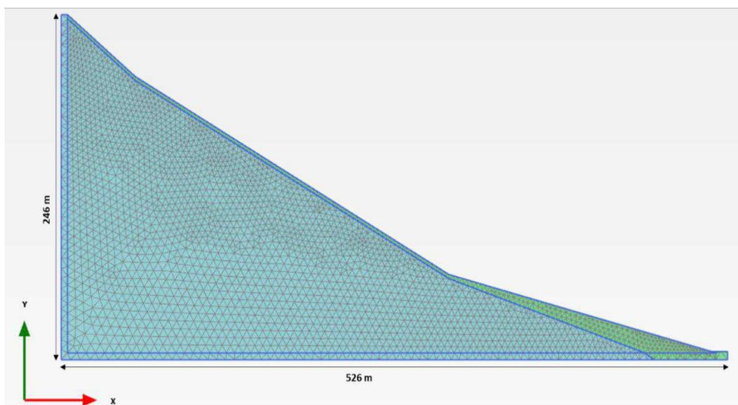
**Fig. 4.14:** Finite element mesh discretization of slope considered
