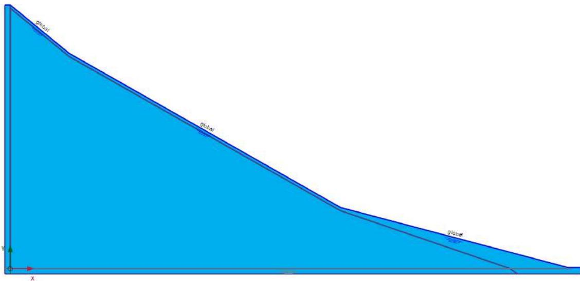
**Fig. 4.18:** FEM model, the water level at the bottom of the slope (fully saturated) - Case 3
