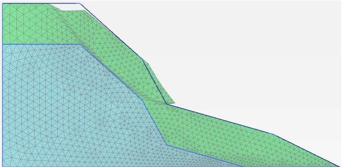
**Fig. 4.26:** FEM model, deformed mesh shape at the time of failure (fully saturated) – Case 3 ( $FoS < 1$ ) for Munnar Silent Valley Road site (LS1)
