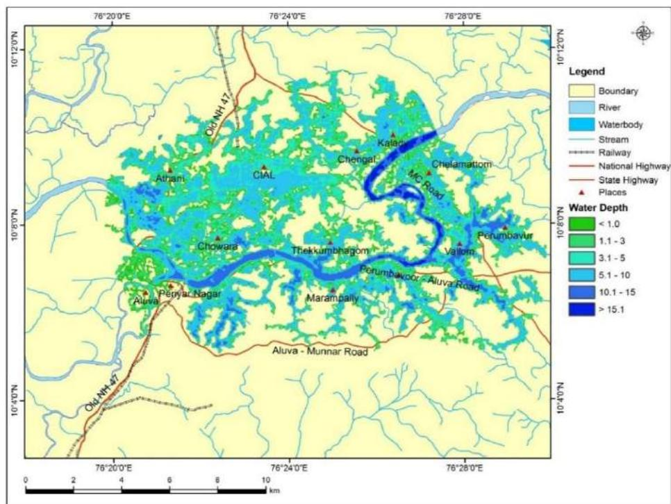
**Fig. 5.10:** Map showing the maximum depth of inundation corresponding to a 24h 100-year rainfall with an initial storage of 75% in the reservoirs
