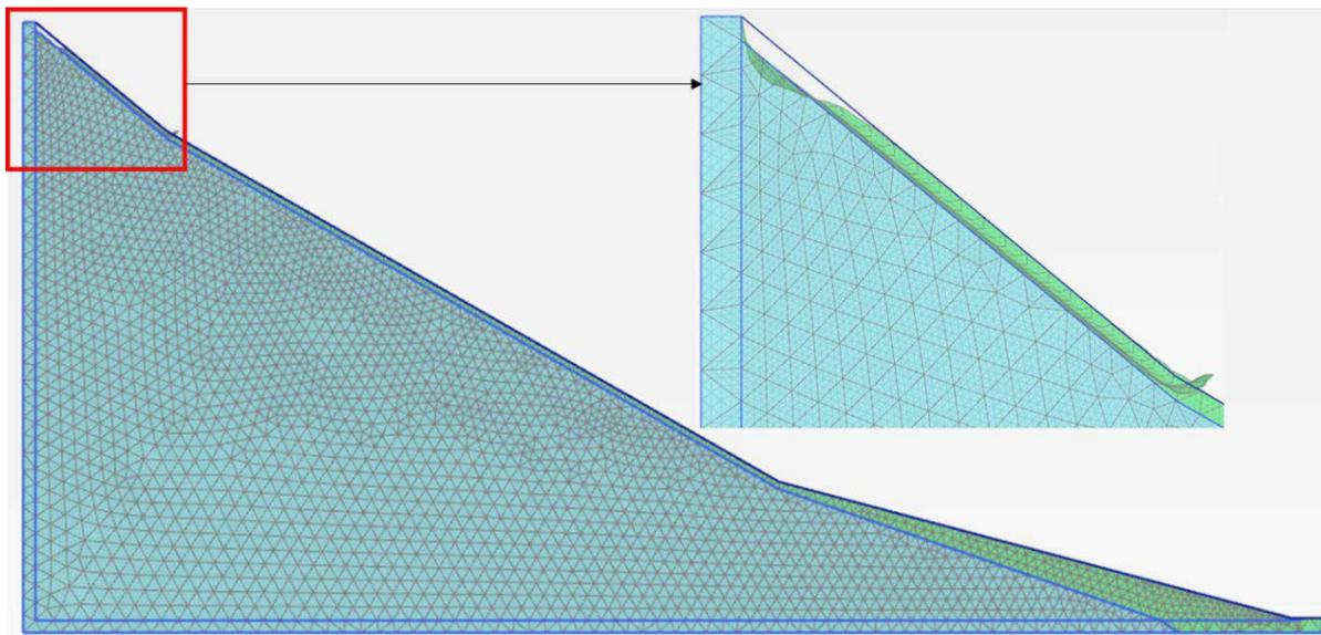
**Fig. 4.20:** FEM model, deformed mesh shape at the time of failure (fully saturated) - Case 3
