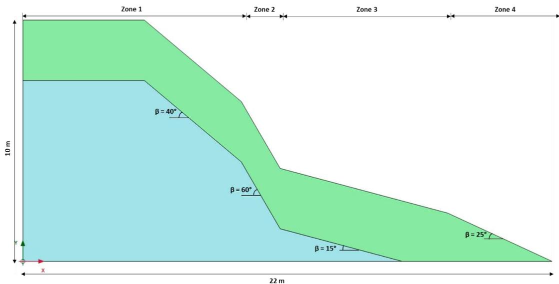
**Fig. 4.22:** Input geometry of slope in the numerical model at Munnar Silent Valley Road site (LS1)
