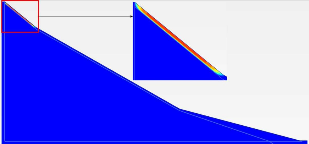
**Fig. 4.19:** FEM model, incremental displacement contours at the time of failure (fully saturated)
