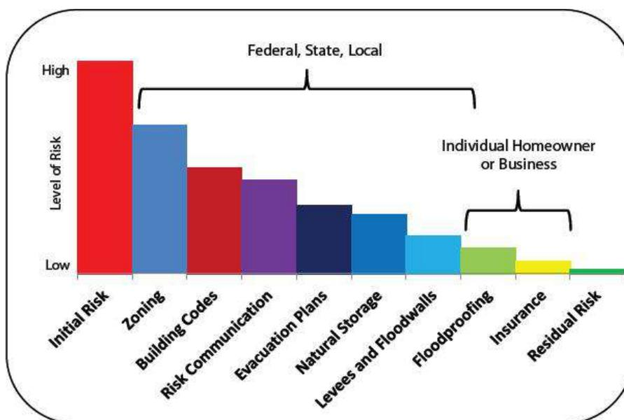
**Fig. 5.23:** Examples of tools and measures to reduce and transfer flood risk in flood-prone areas
