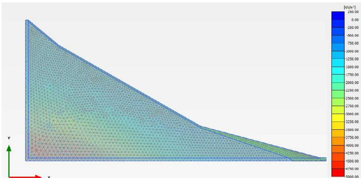
**Fig. 4.16:** Estimated geostatic stresses ( $\sigma_{yy}$  - vertical effective stress) in the FEM model – Initial phase for Kavalappara landslide site
